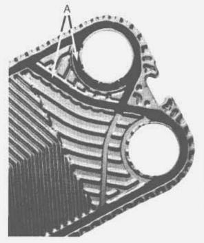
The Sonder Safe plate pair system gives as the only double plate an extra safety by the design of the double plates with leak channels to the atmosphere. This ensures an instant and readily visible trace of possible leaks as a warning that corrective actions should be initiated.
